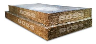
BOSS Party Wall Batts comprises a one-piece, close dimensioned rockwool having a structural internal mineral fibre core. The product has integrated aluminium foil facings to provide class 'O' rating and excellent resistance to smoke. A unique method of manufacture provides a resilient lateral compression required to ensure a tight fit. Designed to be used in Ceiling Cavity, Slab Edge or Under Floor installations and upgrades.
