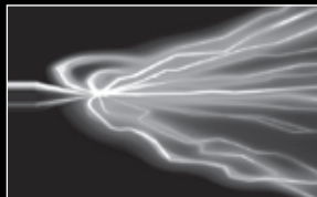
The streamer discharge generates high-speed electrons.
