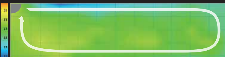
For the 5.0 kW model, the airflow distance is 12 metres 2 . The time required to reach the set temperature is only half of that for a conventional Daikin inverter model 3 for the Japanese market.
