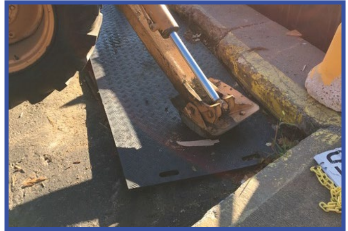
Stabilization Reusable traction and support for vehicles and equipment
