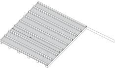
g LMAX crewing 4 Install the batten on top of the COOLMAX foil according to the roof tile manufacturer's recommendations.
