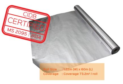
The CoolMax MS AWA K750 (Product Code: CF2A FR), consists of 5 layers laminate made up of double sided aluminium foil, bonded to reinforce high density polyethylene woven fabric by special tie layer bonding material.
