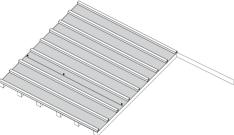
4 Install the batten on top of the COOLMAX foil according to the roof tile manufacturer's recommendations.
