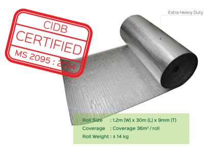
**The CoolMax TRIPLEX FR NET (Product Code: CPM5 NET )**, is made of 2 external pure aluminium foil, covering a double layer of fire retardant polyethlene bubble film, and a single core layer of XPE fire retardant foam. Emissivity is low (0.03 to 0.05 for each reflective surface), and it is reinforced with bidirectional fiber net. The aluminium thickness are 9 micron for top layer, and 18 micron for bottom layer respectively.
