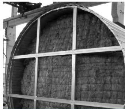
Industrial furnace insulation
