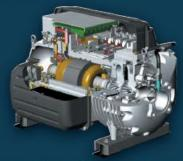
Proprietary magnetic bearings replace conventional oil-lubricated bearings, eliminating high friction losses, mechanical wear and high-maintenance oil management systems. This contributes to the delivery of chiller energy savings of 35 percent and more over conventional chillers whilst ensuring long-term reliability.
